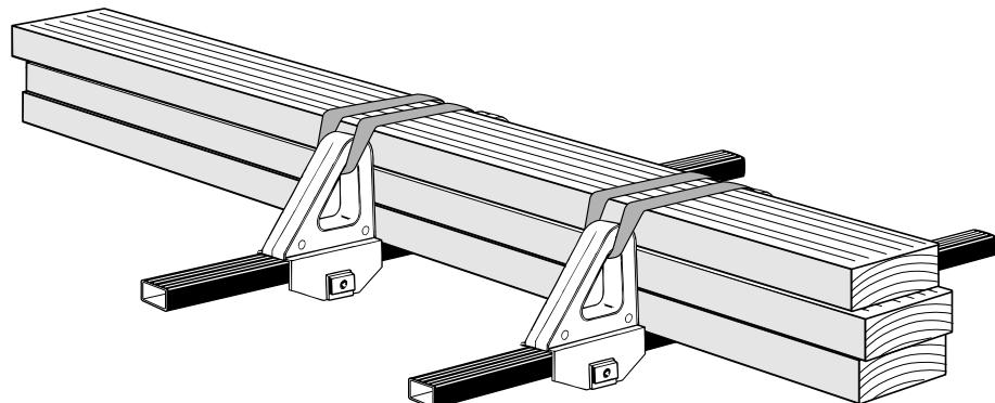
If payload is above level of loadstop secure as shown.
