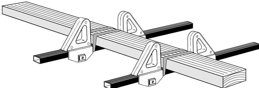
If payload is below tops of loadstops secure as shown.
